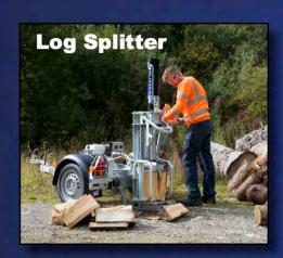
25t splitting ram powered by an on-board petrol engine. Horizontal or vertical splitting. Capacity of up to 600mm length.
