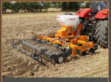
The **Rehab** is a specially designed low surface disturbance subsoiler for both arable and grassland applications.
