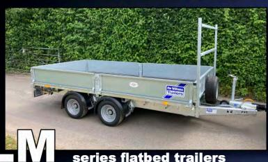
This range of trailers offers platform lengths from the 8ft LM85 up to the 20ft LM208. All are built around a welded steel galvanised chassis with bolt-on taper drawbars. Tri-axle options are available on the larger trailers.
