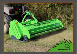
The Ri DS series - a heavy duty double skin flail mower for tractors up to 140hp. Adj rear roller and hyd side shift fitted as standard.
